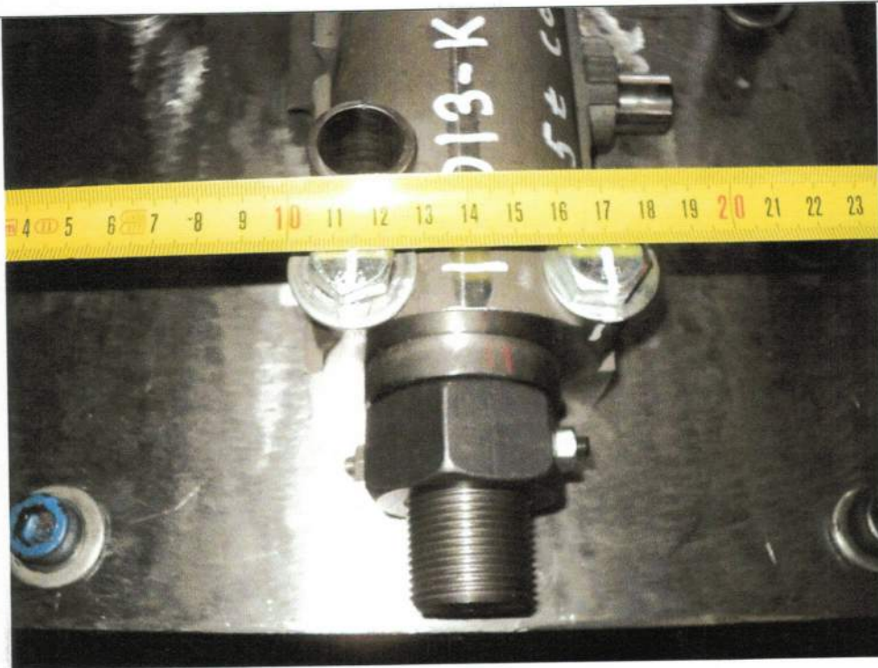
Figure 3: Close up view indicating the critical dimension of the test specimen
