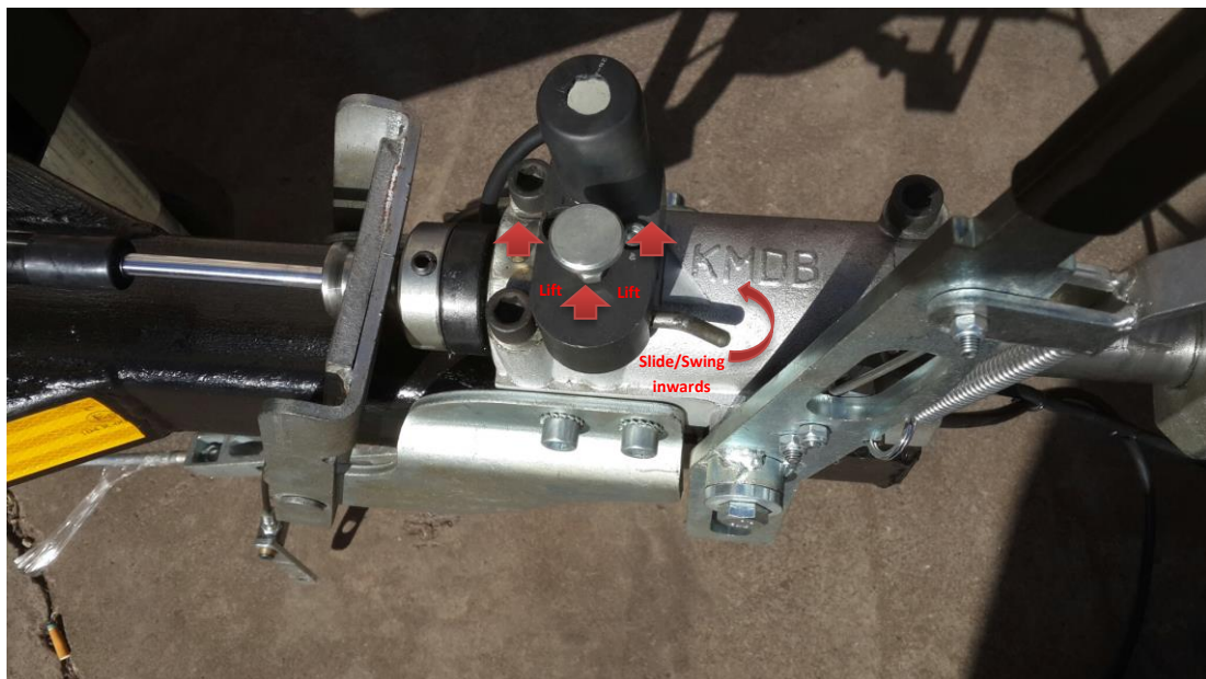
Fig 1. Pull the lock pin up(as illustrated) and swing the manual reverse lever inwards to engage the reverse system manually.
